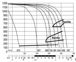
Continuous cooling transformation curve Hardening Temperature 1150°C
