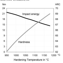
Original dimensions 9 x 12 mm Tempering 3 x 1 hour at 560° C Unnotched test piece 7 x 10 x 55 mm
