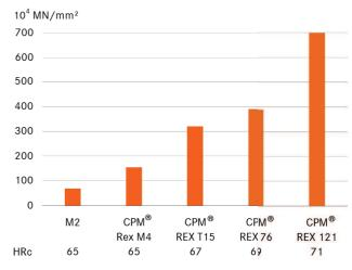
Reciprocal of wear rate in wear test with non lubricated crossed cylinder in contact with a
