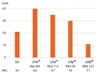
Standard size of the Charpy-test-piece with a 12.7 mm notch radius.
