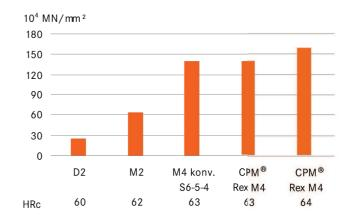
Reciprocal of wear rate in wear test with non lubricated crossed cylinder in contact with a rotation tungsten carbide cylinder.
